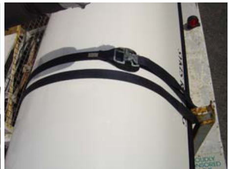
Buckle too high Wrong!
